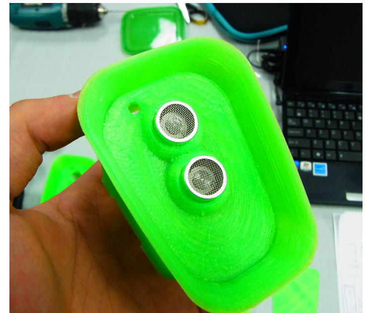
Housing 03 with SRF04 ultrasonic sensor
