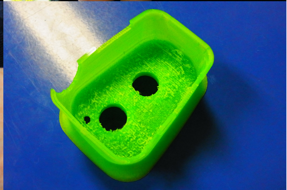
Cleaning up support material from the inside of Housing 02
