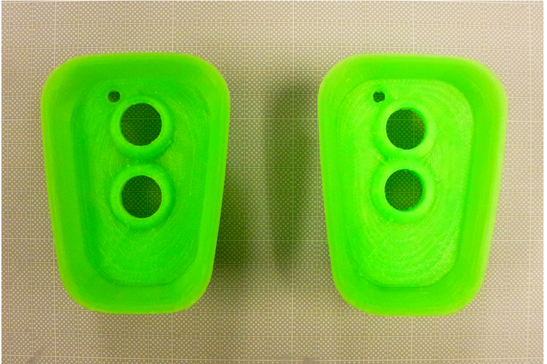
Comparison of Housing 02 (left) and Housing 03 (right). The space between holes suit the different ultrasonic sensors
