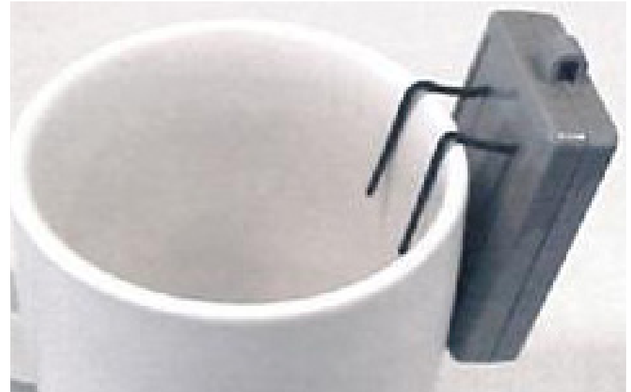
Liquid Level Sensor from Vision Australia Store, item code: ES7271
