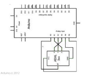
Accelerometers can be bought presoldered to a PCB. This saves you the burden of soldering the required auxiliary components. The PCB with the accelerometer on it can simply be connected to an Arduino as shown to the left. Note that this example uses analog pins as power and ground. These pins are then defined as such in the Arduino code (see next page). For elaboration click here.
