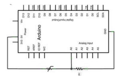
Again, this circuit uses same basic voltage divider principle used in previous chapters to produce varying voltage outputs, in this case in relation to temperature "felt" by the thermistor. Use 10KOhm for R1 (if you're using a 10KOhm thermistor).
