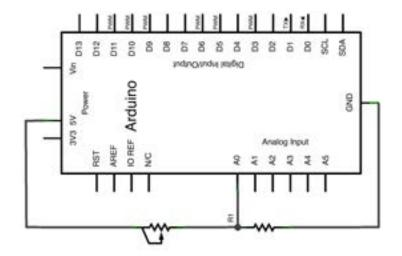
This circuit shows the force sensitive resistor configured in a voltage divider in order for the force applied to the sensor to influence the output voltage read by the analog Arduino input. Note that this exactly the same circuit as in the voltage divider chapter, but with one of the regular resistors swapped for the force sensitive resistor. Use 10KOhm for the remaining resistor.
