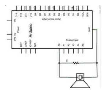
As explained on the last page, piezoelectric elements generate small charged when deformed. In the circuit on the left these charges are fed into the Arduino's analog input to be measured. Use a 1MOhm resistor for R1. For elaboration click here.
