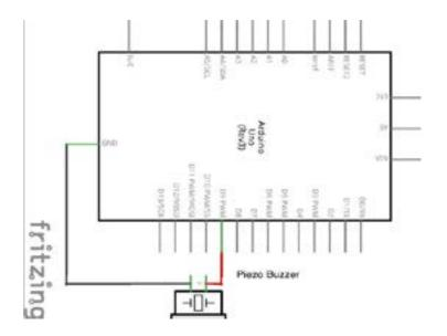
This circuit diagram shows that you connect the positive lead (read) of the piezo buzzer to digital pin 9 of the arduino and the negative lead (black) to the ground (GND) pin of the arduino.
