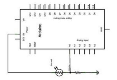
This circuit shows the LDR configured in a voltage divider in order for the light intensity on the sensor to influence the output voltage read by the analog Arduino input. Note that this exactly the same circuit as shown in the voltage divider chapter, but with one of the regular resistors swapped for an LDR. Use 10KOhm for the remaining resistor.
