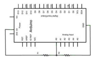
This circuit diagram shows a voltage divider wired so that the regulated output voltage can be read by the analog input of the Arduino. Feel free to play around different resistor values to get different outputs.
