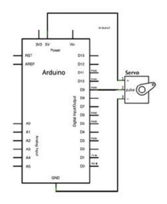
This diagram shows that you connect the 5V pin to the positive input of the servo (1), the digital pin 9 to the pulse input (2) and the negative of the servo to the ground pin of the arduino. You will notice that the power does not come from the digital pin as it is used to send/receive information on servo positioning. Review the code for this on the next page.
