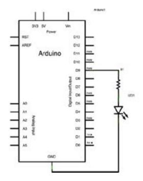
This circuit diagram shows that you put a resistor in series with an LED between the digital pin no. 9 and the ground. It is important that you use a digital pin with pulse width modulation or PWM. This means you can declare any of the pins with PWM. If you'd like to change which pin to plug the resistor and LED combination into. Review the code for this on the next page.
